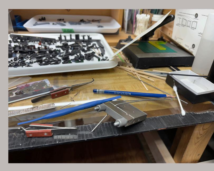
In this photograph the wire has been clamped in the brake and the wire is being bent to the desired angle. you can see a 90 degree bend has already been made in the other end of the wire.
